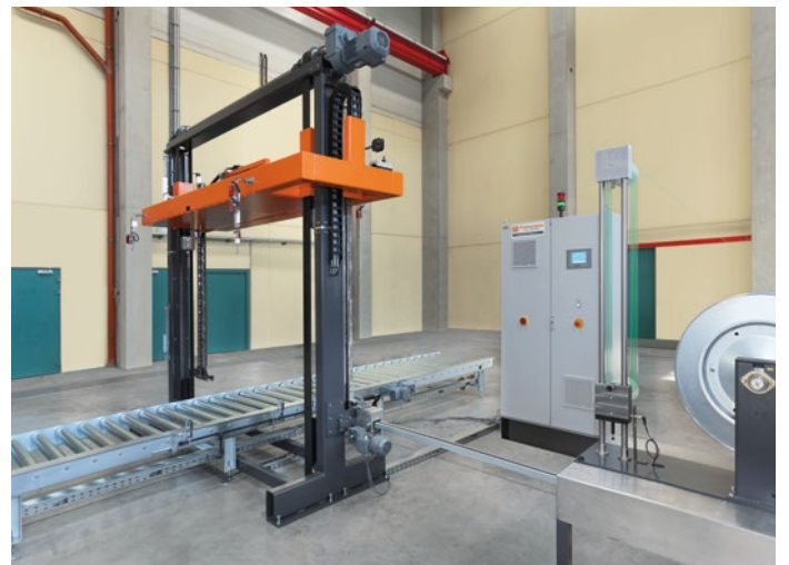
V Strapping machine: Vertical strapping machine with sealing facility at the top of the pallet for IKEA, Sweden.
