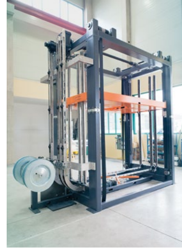
Strapping press for 5 tons pressing force Made in Austria.
