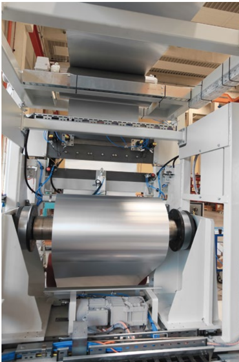
Coiling system for film production - Solar cell manufacture.
