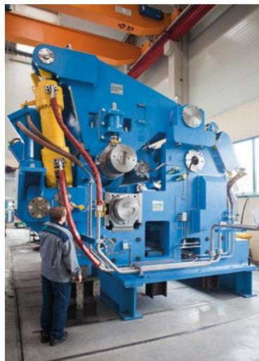
Driver for hot rolling mills - 64 tons of piece weight.
