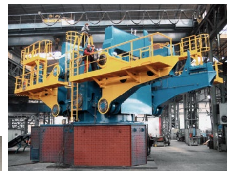
Ladle turret for a continuous cast slab plant.
